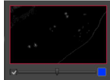
**Blue frame** rectangle indicates displaying of already recorded filter set image. The recorded image is activated and displayed on the image main window of GRYPHAX software. The image parameter of Fluorescence tool are deactivated.
